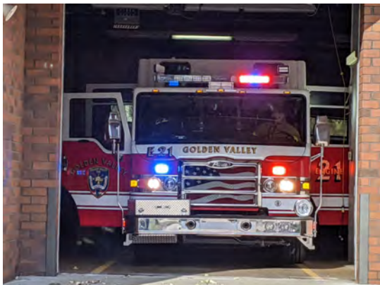
Fire Department: Figure 4 Building Limitations Fire Station #2 with Engine 21: the existing garage bays were designed at a time when apparatus were smaller. As shown in the photograph, current bays are not sufficiently wide enough, causing issues with back-in parking (potential vehicle and structural damage) and with turn-out after firefighters return to the station - i.e. removal of firefighting gear and equipment.
